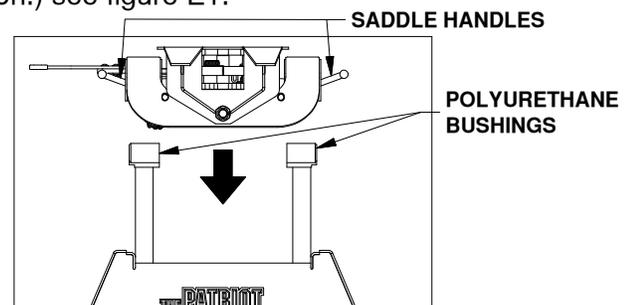
FIGURE E1: View of coupler and base. (Saddle Handles up)
