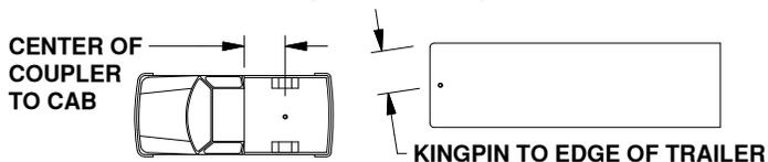
**⚠ WARNING:** Check the clearance between the bed side and the underside of the front of the trailer and to allow adequate clearance for the pitch and roll of the trailer while towing.
