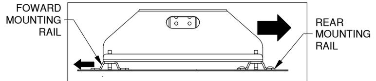
Figure E2: Side view of RV base and mounting rails.
