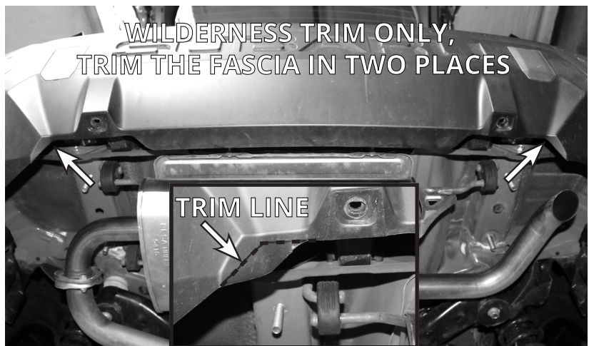
FIGURE B1: VIEW UNDER THE REAR OF THE VEHICLE
