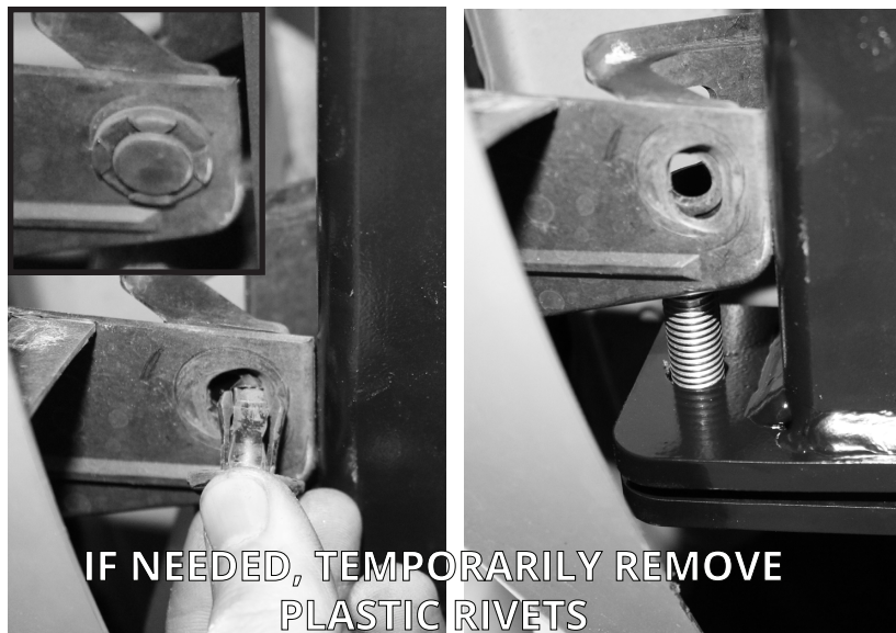
FIGURE C3: VIEW UNDER THE REAR OF THE VEHICLE
