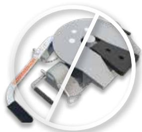
Preventing the kingpin from rotating within the jaws of the Companion coupler with a wedge, or any other device, such as Reese Sidewinder® or Reese Revolution®, could result in property damage, serious injury or death.
