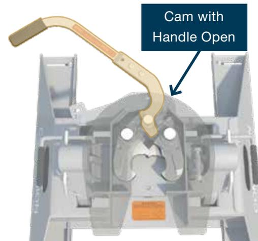
When the handle is open the cam allows the jaws to open, even if you are in a bind because of unlevel ground. If the handle is open, you may go ahead and drive out of the jaws. They will open as you pull away.
