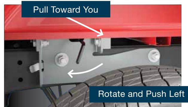
4. Remove the base. Use the ball, in the inverted position, to fill the receiver hole when not towing.
