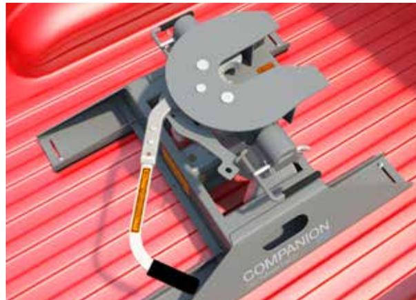
4. Ensure that the coupler cam handle has completely closed and insert the cam handle safety pin through the cam handle and the coupler.
