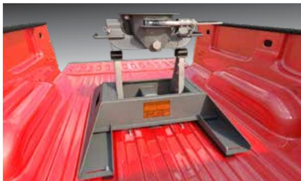
2. Swivel the locking bracket from over the drawdown bolt head. Loosen the drawdown bolt.
