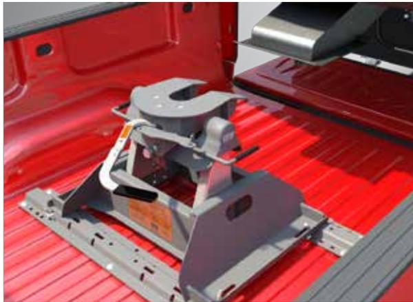
2. Adjust the height of the fifth wheel trailer using the jack so that the kingpin plate is slightly lower than the top of the coupler.
