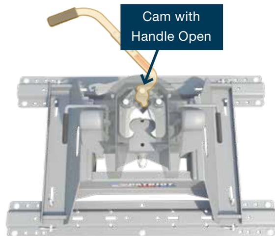
When the handle is open the cam allows the jaws to open, even if you are in a bind because of unlevel ground. If the handle is pinned open, you may go ahead and drive out of the jaws. They will open as you pull away.
