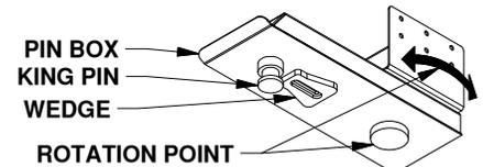
Figure F2: Pin box with rotation point.
