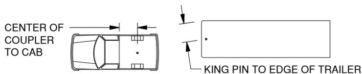
**WARNING:** B&W also recommends that you check the clearance between the bed side and the underside of the front of the trailer and to allow adequate clearance for the pitch and roll of the trailer while towing.
