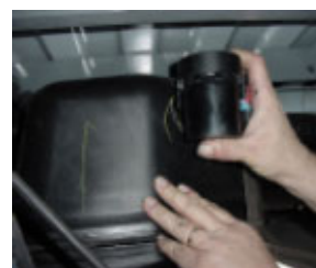
Figure C3, Step 3: Slide fuel valve from bracket.
