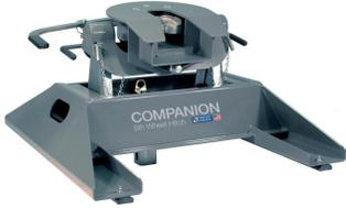
3. We design a hitch that fits newer model trucks that have the 4 holes already drilled in their truck bed. These holes with pucks are drilled at the truck factories and only work with specific hitches. Be careful before buying a truck with this system, because it may limit your choices. [The Companion OEM 5th Wheel Hitch.](#)
