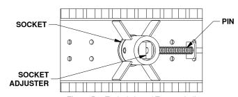
Figure B2: Typical view of Turnoverball gooseneck center under bed.
