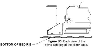
**NOTICE: Nissan Titan trucks:** Due to the configuration of the bed ribs on Nissan Titan trucks, it will be necessary for the foot pad positioned on top of a bed rib.
