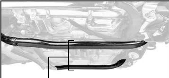
Distance from the outside edges of each frame tube must be no less than 10" and not more than 14.5". Take this measurement where the Biker Bar will be attached.
