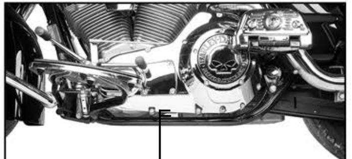
There must be 1/2" of clearance between the motor, transmission, and the primary drive to allow clearance for the Biker Bar clamps.
