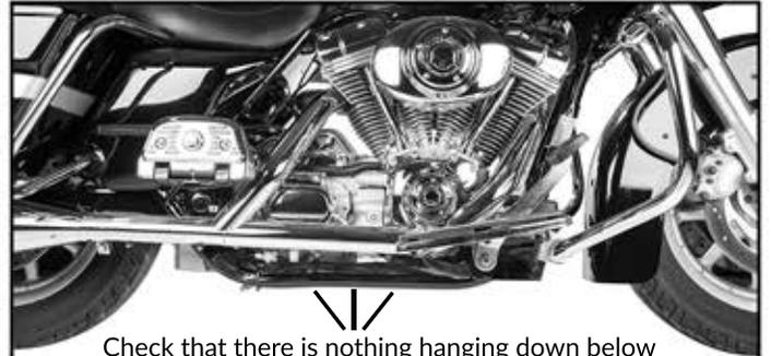
Check that there is nothing hanging down below the tube frame, such as a motor, transmission or exhaust. With the rider sitting on the motorcycle, the distance from the side of the frame tubes to the ground must measure between 5" & 6.5".
