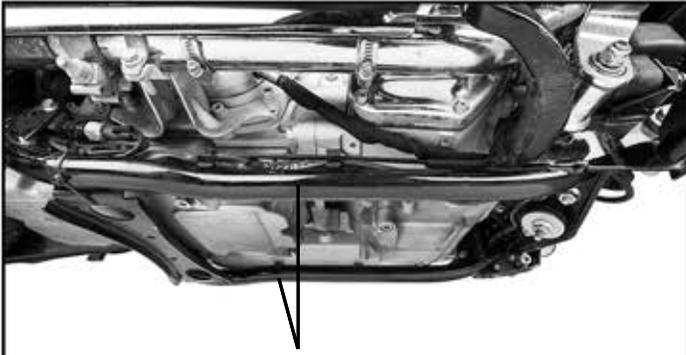
A two piece motorcycle tube frame is needed for the Biker Bar to clamp onto. The diameter of each frame tube must be at least 1.125" and no more than 1.5"
