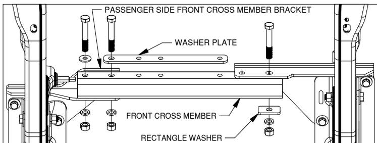
Figure C3: Bottom of truck frame looking up from under the cab towards the back of the truck.
