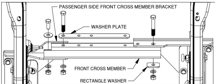
Figure C2: Bottom of truck frame looking up from under the cab towards the back of the truck.
