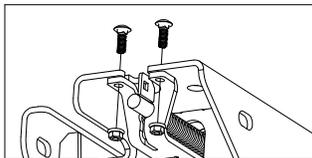
Figure C3: Latch pin assembly (short bed installation).
